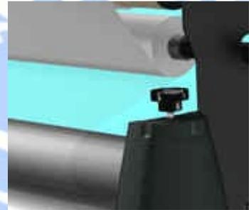
Two knobs set the height and pressure of the top roller.
