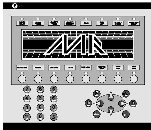
indication. Based on your pre-determined Message and Error code listing, enter the corresponding code number, then press the "ENTER" key. Your selections are now saved in the PLC memory.
