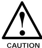
**CAUTION:** The new battery must be connected within five minutes of removing the old one to preserve the data in the PLC.
